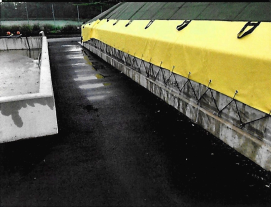
CASP SYSTEM: COVERED AERATED STATIC PILES - Feedstock is covered in a concrete bunker system process, creating a closed system that fully contains leachate and minimizes odors.
